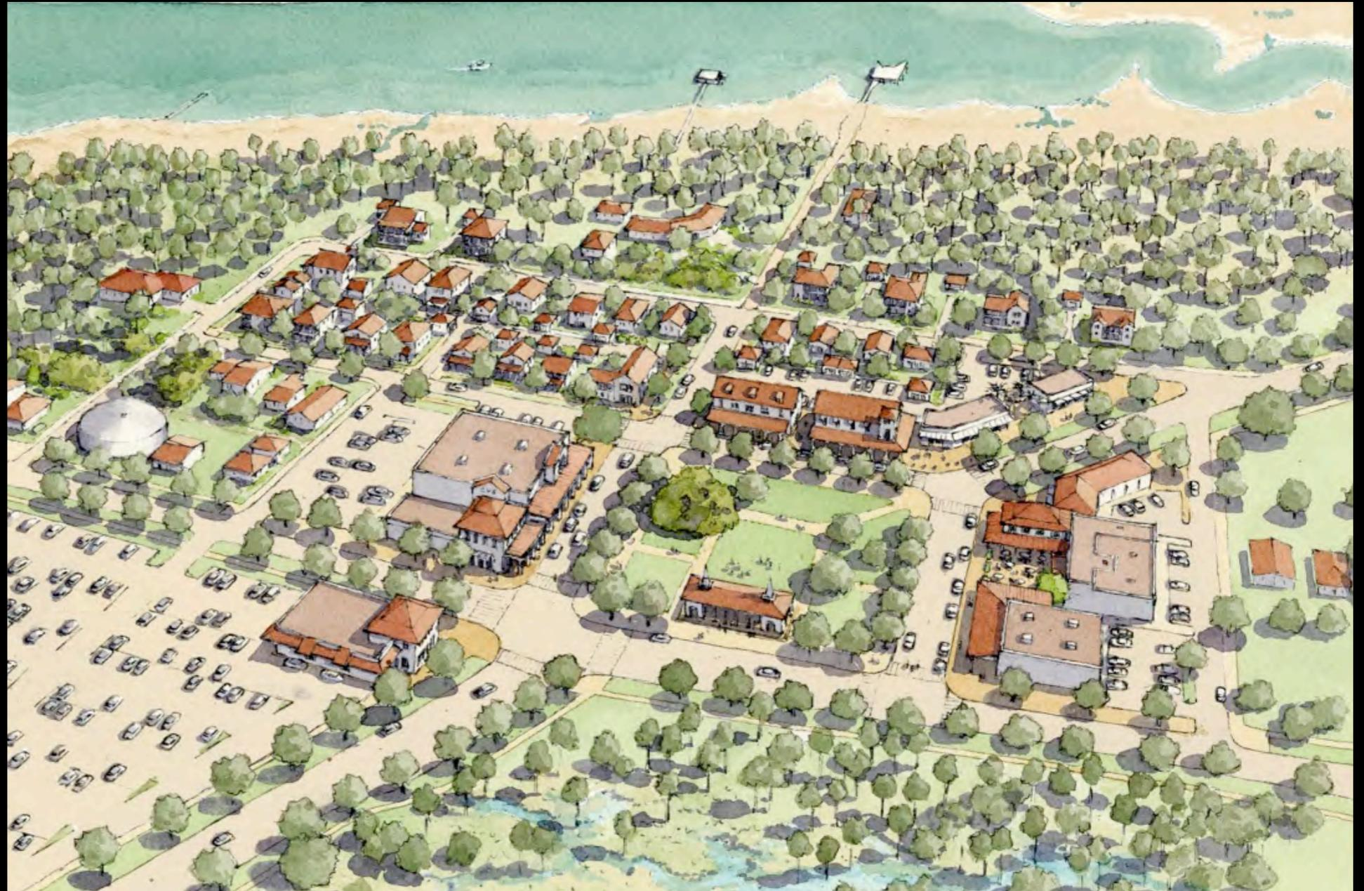
The new square-about with a civic building at the center of the intersection keeps the flow of traffic unimpeded, as the 4 lanes of Perdido Key Drive are kept to distribute drivers around to Sorrento Road, Innerarity Road and Gulf Beach Highway, yet it divides those lanes into two faster and two slow ones; the latter running next to parallel parking along the wide sidewalks of cafes and restaurants. The
